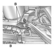
Lift the vehicle with the jack, making sure the jack spans at least two of the crossmember ribs (B).
